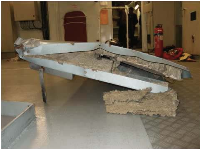
Fig. 20: Steel Door from Harmonic Filter Capacitor bank on Queen Mary II REF SB4-10
