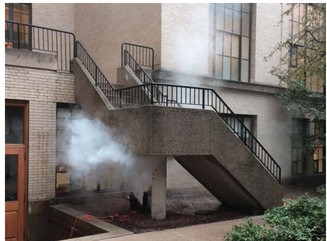
Fig. 15: Small Scale Test showing destruction of DC link capacitors
